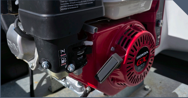
Water Pump Honda GX160 Semi trash water pump - 1000Lpm 28m max head.
