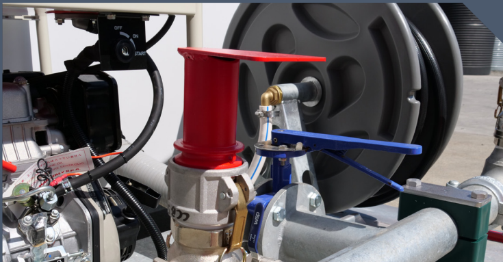
Spray Nozzles 3 x 2" rear batter sprays nozzles set by flow adjustable brass ball valves. Rear sprays fully adjustable with 360 degree rotation.
